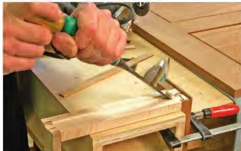
Hidden away. The hidden drawer rides on wooden slides attached to the carcass. The end of the groove will act as a stop for the runners, and needs to end in the right spot.
